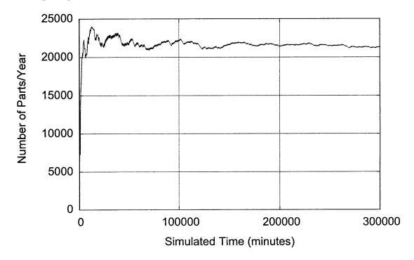
Figure 11: Production rate vs. time with proposed polishing improvements and a single worker with a demand rate of 25,000 parts per year.
