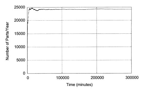
Figure 5: Production rate over time of the existing production system. Demand rate is 30,000 parts per year.
