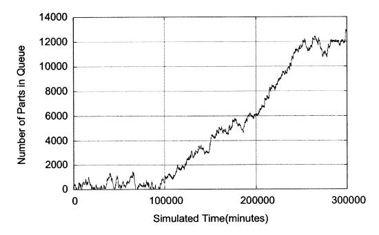
Figure 10: Queue length over time for the grinding node at a demand rate of 48,000 parts per year.
