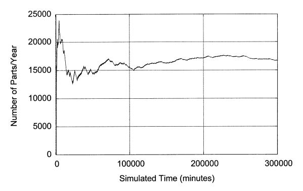
Figure 12: System production rate with a 15% rework rate at the buffing stage.
