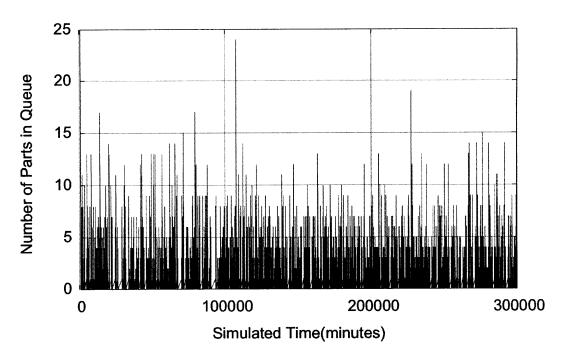
Figure 9: Queue length over time for the bras polishing node at a demand rate of 48,000 parts per year.
