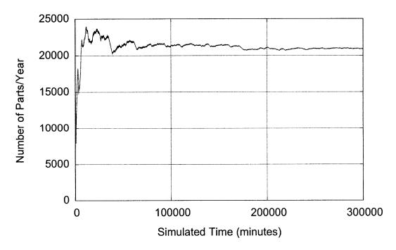
Figure 13: System production rate with a 25% rework rate at the polishing stage.
