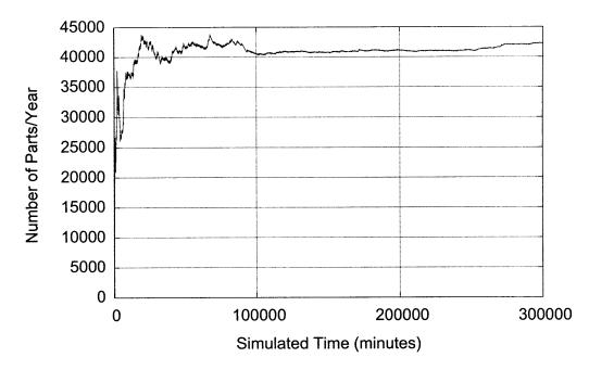
**Figure 8:** Production rate over time with the proposed improvements to the polishing process. Demand rate is 48,000 parts/year.
