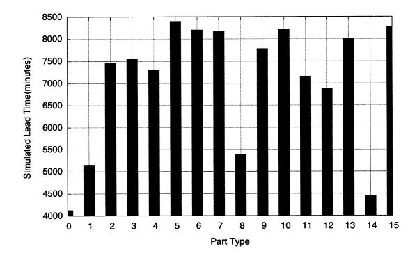
Figure 3: Sample lead time by part type of the existing system. Parts Types 0-7 represent brass parts while 8-15 represent steel parts.
