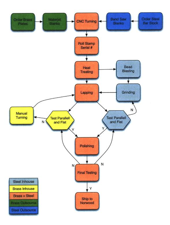
Figure 1: Test Block Manufacturing Process Flow Chart
