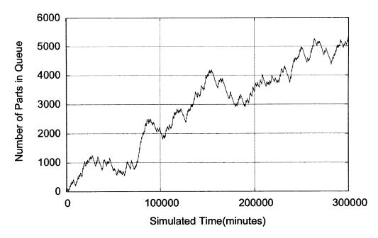
Figure 7: Queue length for the brass polishing node at a demand rate of 30,000 parts per year.
