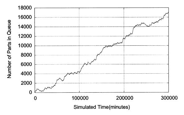
Figure 6: Queue length for the steel polishing node at a demand rate of 30,000 parts per year.
