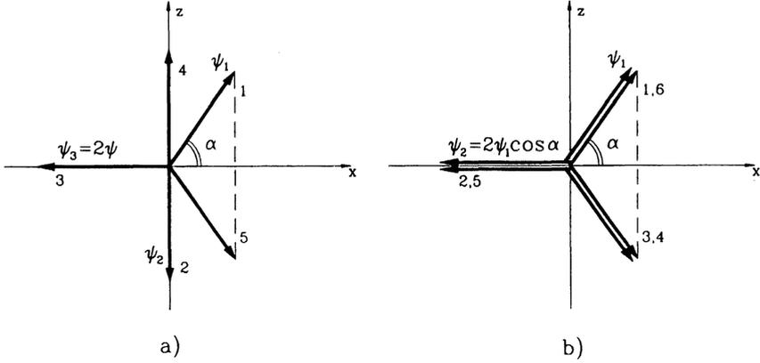
FIGURE 5: Discrete analogues for the helical snakes: (a) five magnet antisymmetric snake; (b) six magnet symmetric snake.
