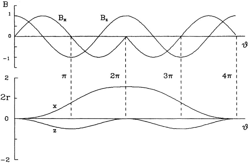
FIGURE 2: Magnetic field configuration and particle orbit excursion profile for the symmetric helical snake.
