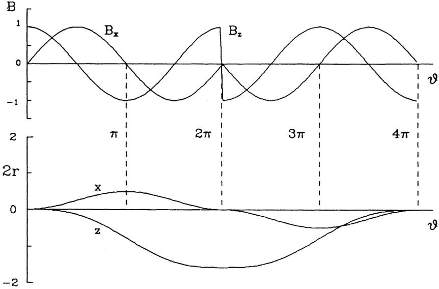
FIGURE 1: Antisymmetric helical snake magnetic field configuration and particle orbit excursion profile.
