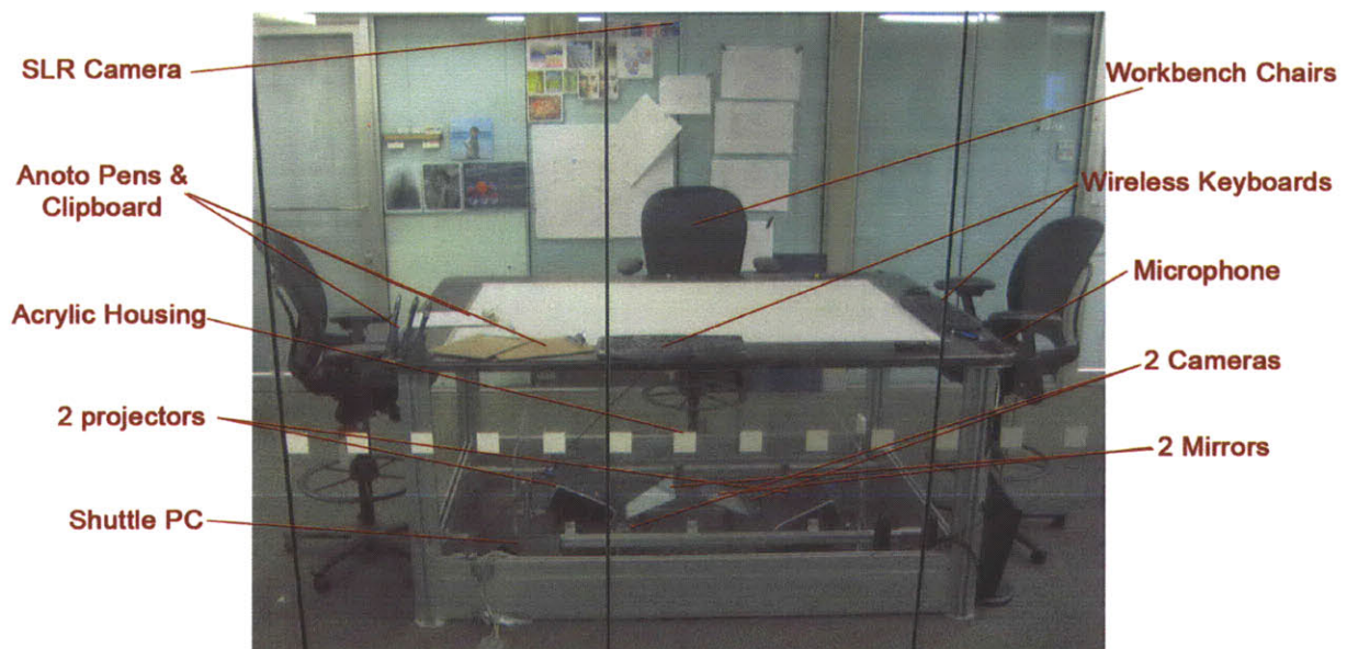
Figure 22a MemTable component diagram with interior technology and exterior input hardware
