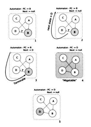
Figure 4.4 – Diagram illustrating automaton migration process
