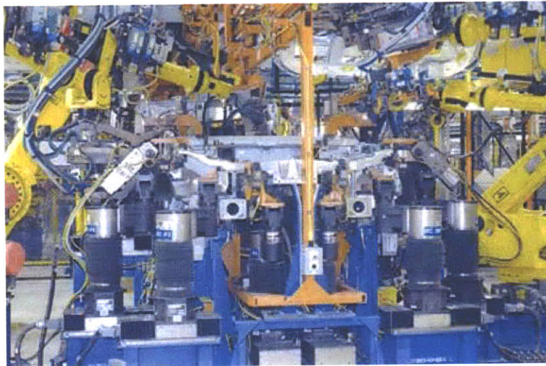
Figure 8 Station comprised of several C-FLEX units surrounded by robots, adopted from (Povelaites 2005)
