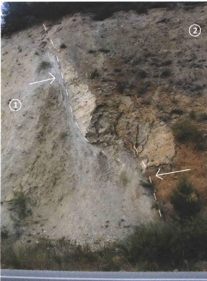
Figure 4-4. Strike-slip fault \alpha_4 Fault plane with NW-SE trending slickenlines separates Marl (1) and Orange Debris Flow (2).
