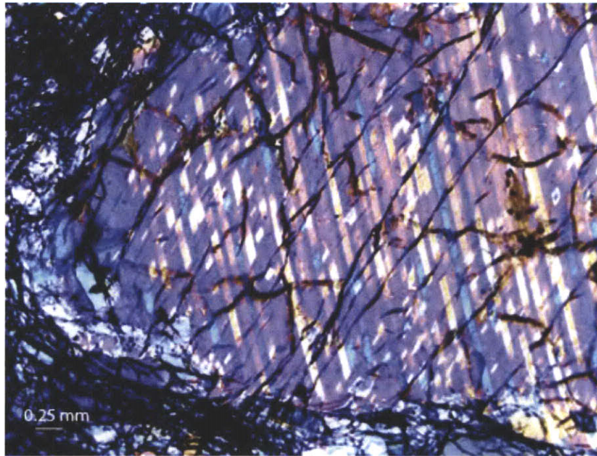
Figure 21. Porphyritic texture in thin section. Large opx egg (purple) shows wide exsolution lamellae of cpx (orange) and is surrounded by small olivine grains.
