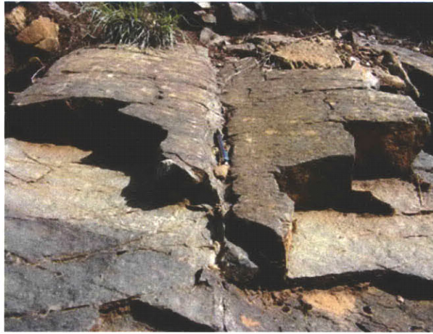
Figure 29. Boudinaged pyroxinite dike. Foliation runs horizontal across picture, and lineation is parallel to the pencil.
