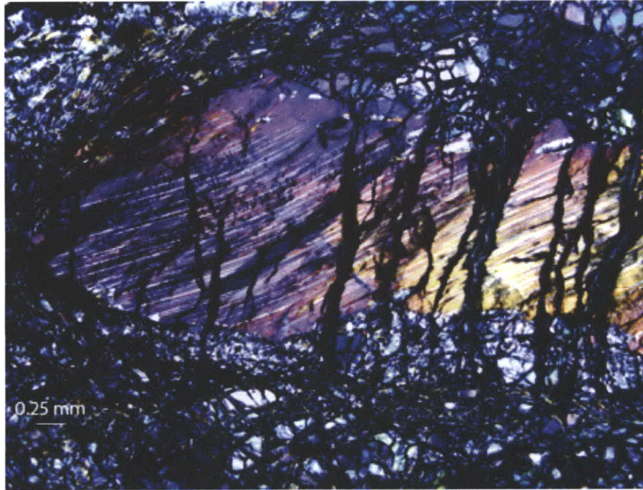
Figure 33. A large, extended opx grain (purple and orange) in thin section showing slightly deformed exsolution lamellae and inclusions of olivine (light blue) at the top of grain.
