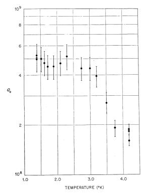
FIG. 6. Unloaded Q,  $Q_0$ , measured as a function of temperature for transmission line position of '4 inch'.
