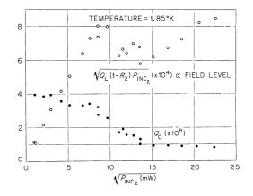
Cavity Filled with Liquid Helium.
