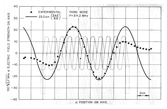
FIG. 4. Axial electric field in second harmonic mode. See Fig. 2.
