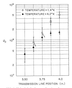
FIG. 5. Unloaded Q,  $Q_0$ , as a function of transmission line position. The horizontal scale is an arbitrary measurement at the top of the dewar. Increasing values of this dimension correspond to withdrawal of the transmission lines.
