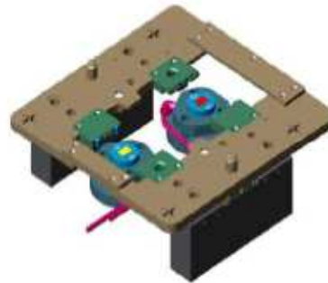
4. Invert turnplate. Repeat for chips 3&4
