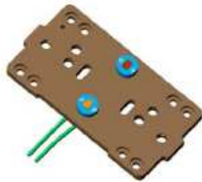
3. Chips transferred and held by vacuum
