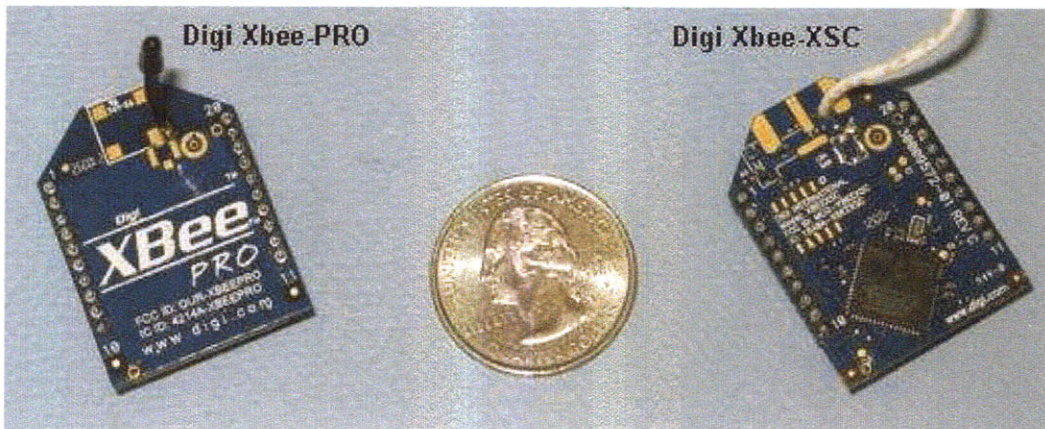
Figure 3-9: The Digi XBee-PRO and Digi XBee-XSC radio modules are used for indoor and outdoor operation, respectively.
