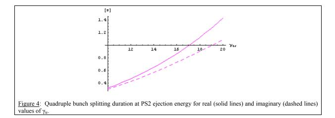
ESME simulations confirm the timescale needed and demonstrate that the voltage requirements of the additional 20 and 40 MHz RF systems for splitting are unchanged from those of the existing hardware. This puts the specification at 20 MHz in the order of a very modest 20 kV.
