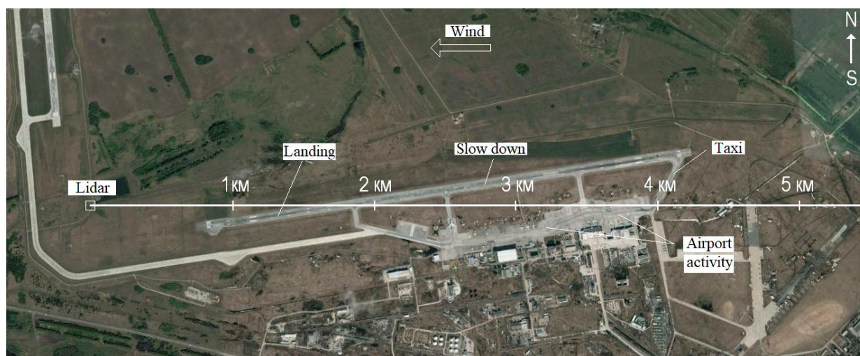
Fig. 2. Tolmachevo airport. The lidar sounding path crossing the run way at 1.5 km. Maximum range is 5 km.
