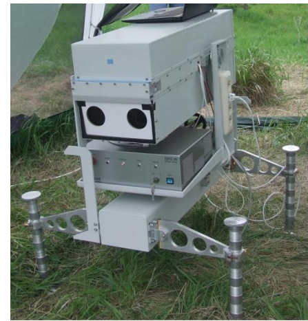
Fig. 1. Optical diagram of turbulent UV lidar (left) and real lidar on the field experiment (right).
