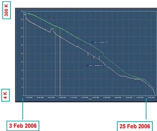
Fig. 2. Graph of the coil minimum and maximum temperatures during the cool-down to 4.5 K.
