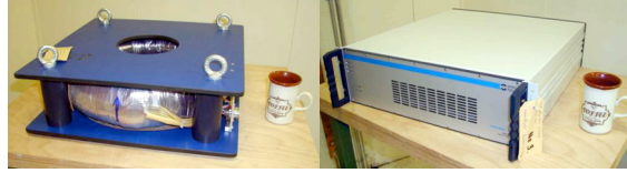
Fig. 16: 13 kA DCCT (head and electronics)
