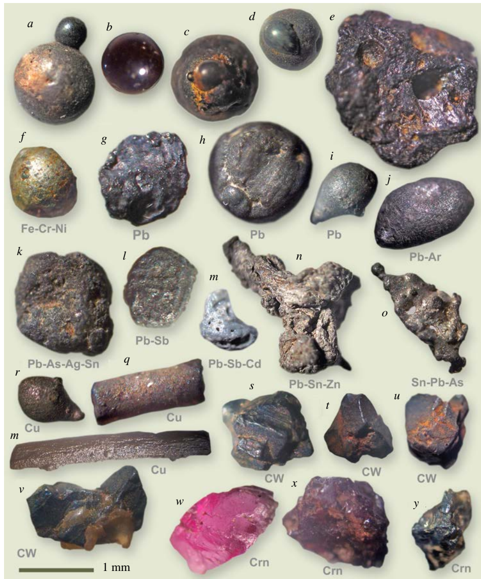
Fig.2. Microphotographs of HRMMA particles from a Mriya lamproite pipe: a-d – TMIS spherules; e – a TMIS glass particle of irregular shape; f-r – particles consisting of native metals and intermetallic alloys ( f-l, p – spherule-like particles, m-o – particles of irregular shape, q, r – rod-shaped particles of native copper); s-v – euhedral crystals of qusongite (WC); w-y – grains of mantle corundum
