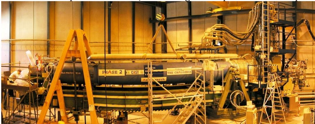
**Figure 35: Positioning of the Expansion Volume on top of the cryostat with the help of the crane.**
