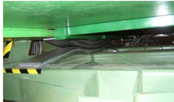
**Figure 48b: Safety cradle installed**
