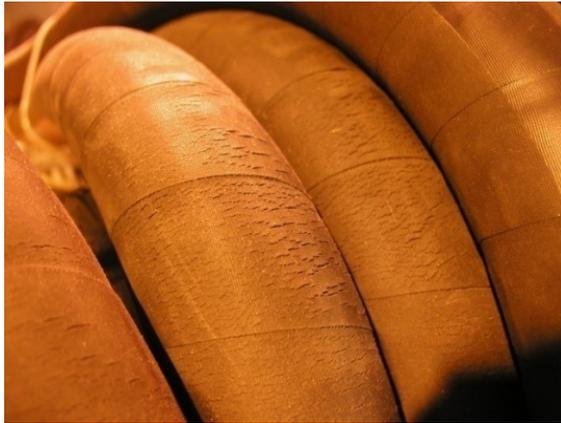
**Figure 49: Aging of the rubber hoses at tip of Potence**
