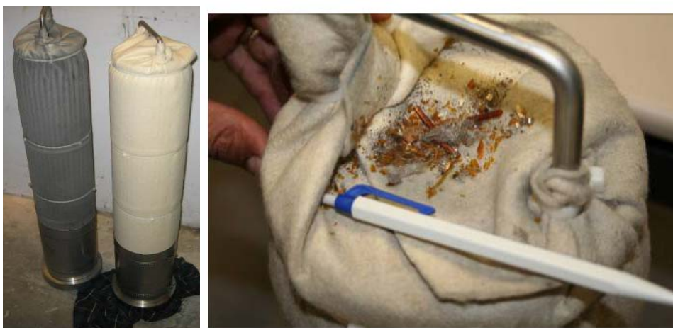
FIGURE 4. Filters after (grey) and before (white) flushing and dusts collected in the filter
