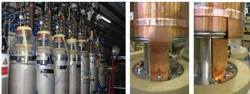
FIGURE 6. Plastic bags with dry air and conduction strips around current lead chimneys
