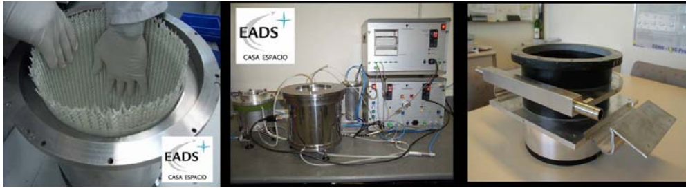
FIGURE 4. Production of GRFE cold mass support posts: assembly of the lay-ups, mould hardware and finished support post equipped with heat intercept flanges.
