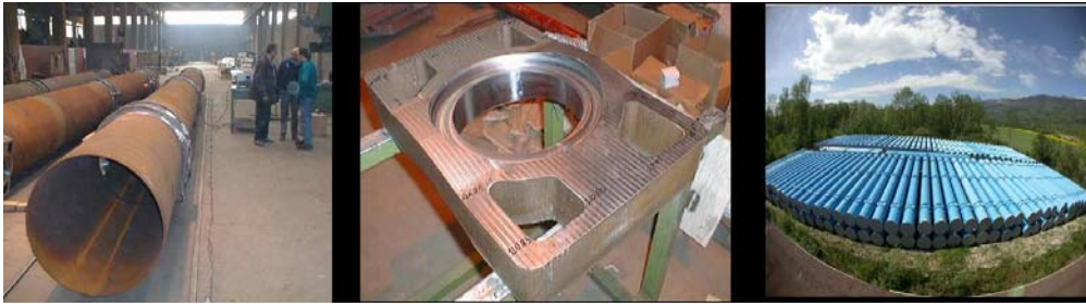
FIGURE 2. Series production of cryostat vacuum vessels : standard tube, forged cradles, and storage of finished vessels.
