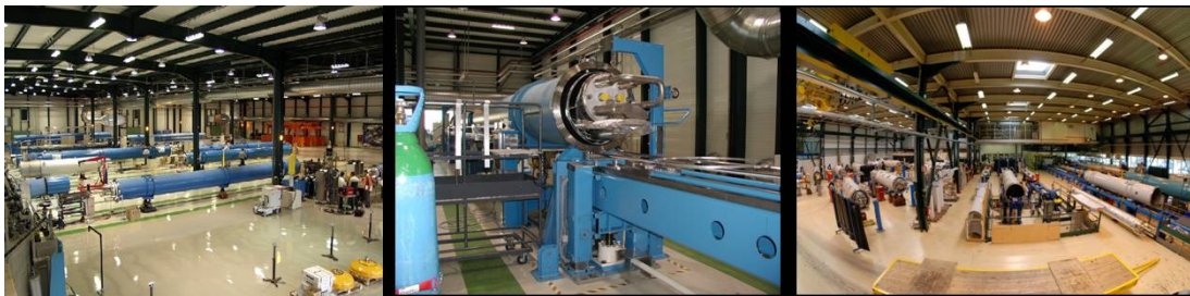
FIGURE 6. Cryostats assembly halls at CERN, and dipole cryostat assembly bench (center)
