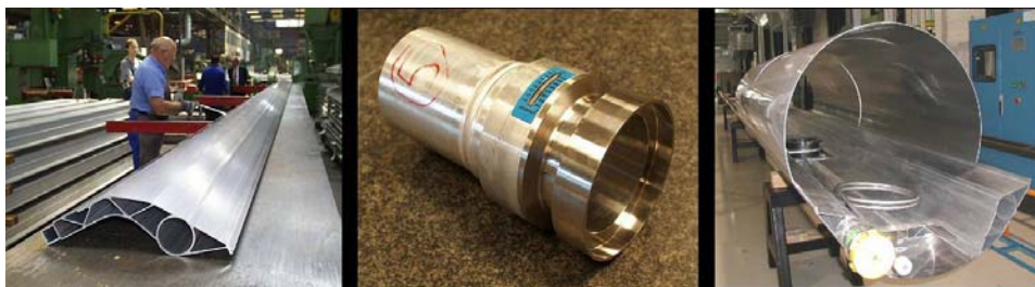
FIGURE 3. Production of cryostat 60 K thermal shield assemblies: extruded profile, aluminium to stainless steel transition, assembled thermal shield.
