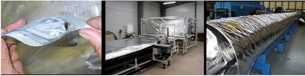
FIGURE 5. Details of large series production of cryostat MLI blankets: lay-up structure, fully automatic blanket assembly table, blankets fitting on a dipole thermal shield.
