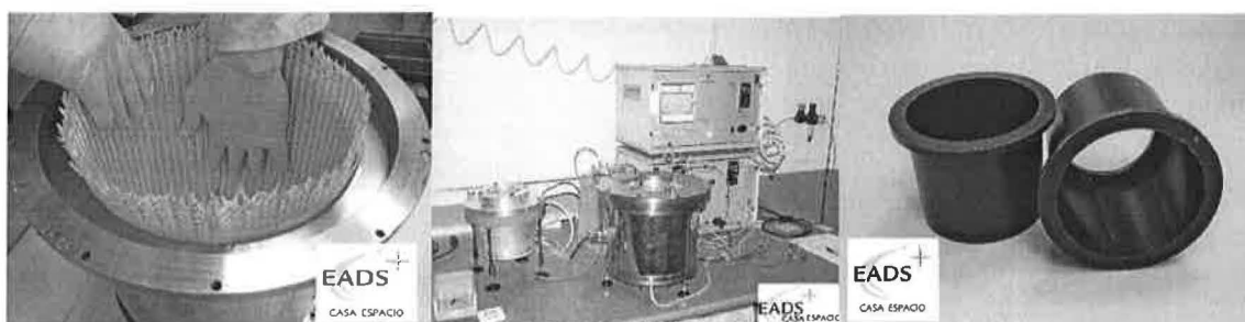
FIGURE 3. RTM process. Stacking of the dry fabrics in the external mould (left); an RTM work station (center); RTM columns after de-moulding (right).
