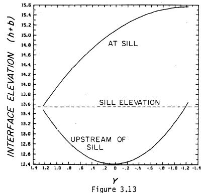
Cross-sectional interface profiles for controlled flow over obstacle with  $b_C/H = 1$ . The flow parameters are the same as those of the upper  $(\phi = .2)$  curve in Figure 3.12.
