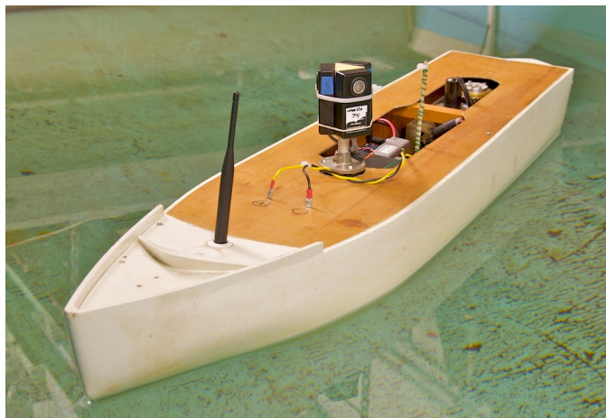
Figure 3-34: The 1.25-meter underactuated surface vessel used in the experiment.
