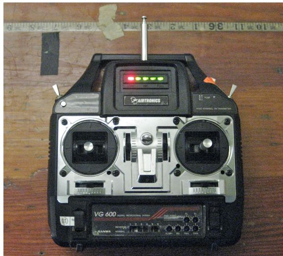
Figure A-5: The radio control transmitter used to manually drive the vehicle. The switch on the upper right corner is used to start the planner and activate automatic control.
