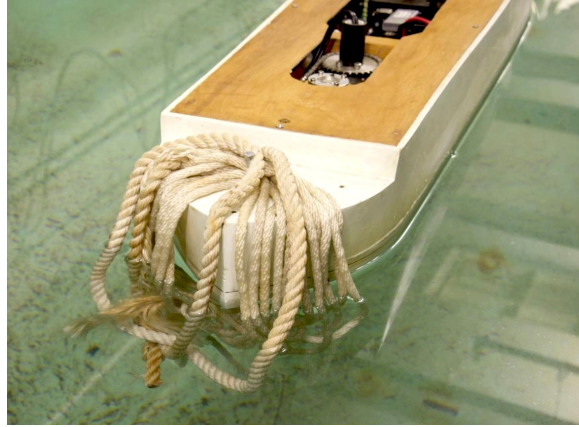
Figure 5-24: Rope was added to the stern of the vessel to increase the yaw drag for the third experiment. The resulting trajectory is shown in Figure 5-25.
