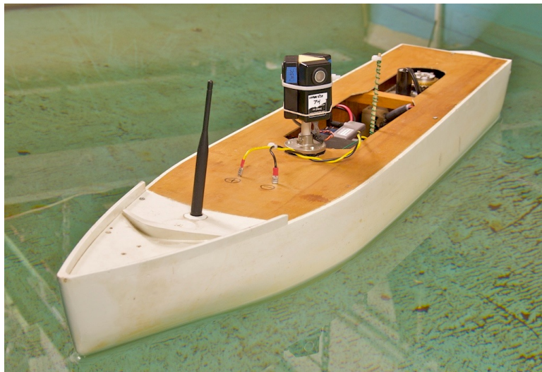
Figure A-1: The autonomous surface vessel used in the experiments. It is a wooden model of an icebreaker. From left to right, the four masts are (1) the radio modem used for the ultrasonic positioning system, (2) the ultrasonic beacons, (3, partially hidden) the computer's wireless router, and (4) the radio control antenna.
