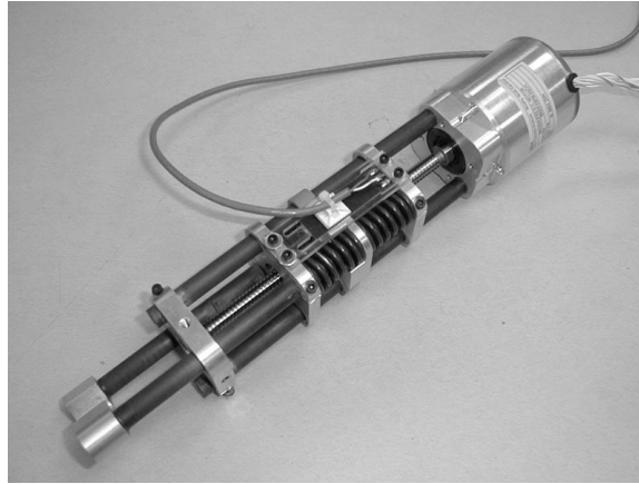
Figure 5-14: EM series elastic actuator used in testing. The actuator uses a brushless DC motor with a direct connection to a 2mm lead ball screw. The ball nut drives the springs in series with the load. The springs are precompressed die compression springs. A linear potentiometer measures the deflection of the springs and uses that signal for feedback to the controller.
