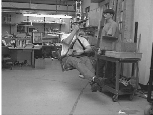
Figure 5-18: Risky testing. The EM prototype actuator is suspended from the ceiling and loaded with 300 lbs (me, seat and weights). The displacement of the spring is commanded so that it compensates for the gravity pull on the load mass. With small variations in the set point, the actuator moves the load up and down.
