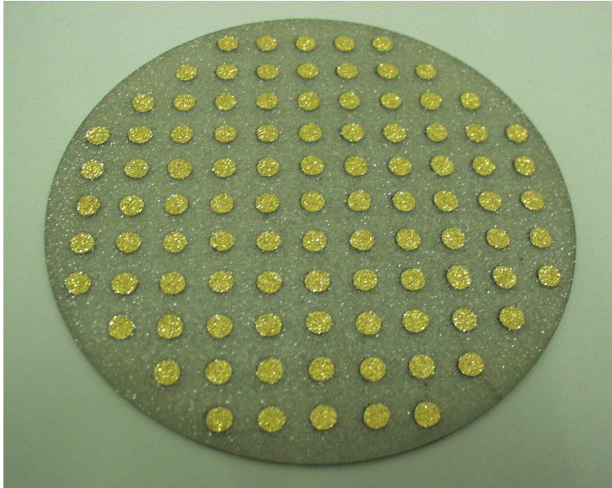
Figure 3. A 13cm diameter wafer of polycrystalline CVD diamond prior to dicing the BCM sensors.
