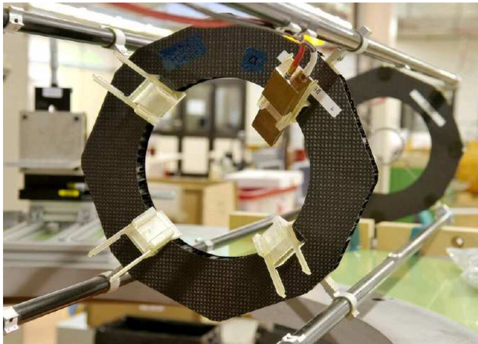
Figure 26. Part of the pixel Beam Pipe Support Structure (BPSS) with the four brackets during a dry-fit of the first BCM module (top right).
