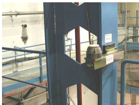
Fig. 5: CERN plug-in reference brackets on wall and on metallic structure with centering socket
