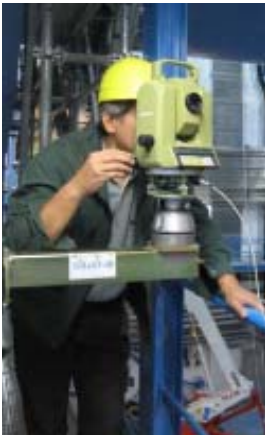
Fig. 30: Station and part of the reference network, Kalman filter basis, USA wall deformation over 3 years.
