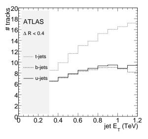
Figure 4: The number of reconstructed tracks  $(p_T > 1, \Delta R_{jet-track} < 0.4)$  versus jet  $p_T$  for ujets (dashed), b-jets (dotted) and top quark with hadronic *W* decay (continuous line).
