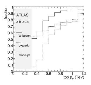
Figure 1: The fraction of top quark decays where the W-boson (continuous line) or b-quark (dashed line) are within  $\Delta R = \sqrt{(\Delta \phi)^2 + (\Delta \eta)^2} < 0.4$  of the reconstructed jet axis versus top quark transverse momentum.
