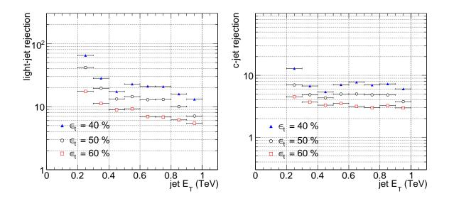
Figure 5: Light jet rejection (leftmost figure) and charm jet rejection (rightmost figure) of the combined *SV1+IP3D* algorithm versus jet transverse energy for three choices of the tagging efficiency for hadronic top *monojets*.
