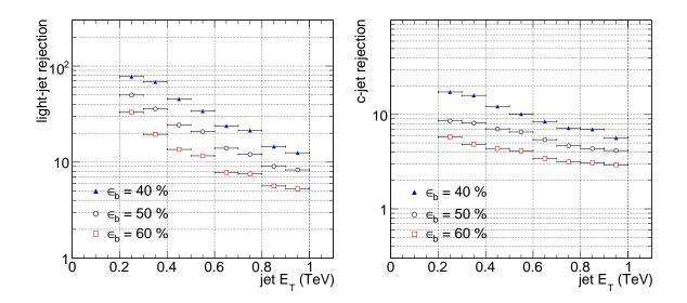
Figure 2: Light jet rejection (leftmost figure) and charm jet rejection (rightmost figure) versus jet transverse energy. The results correspond to the combined SV1+IP3D algorithm after a retuning for highly energetic jets. The three sets of markers represent three choices of the b-tagging efficiency.
