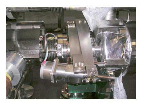
Figure 6.2 Photograph of CTS tuning system attached to the cavity.
