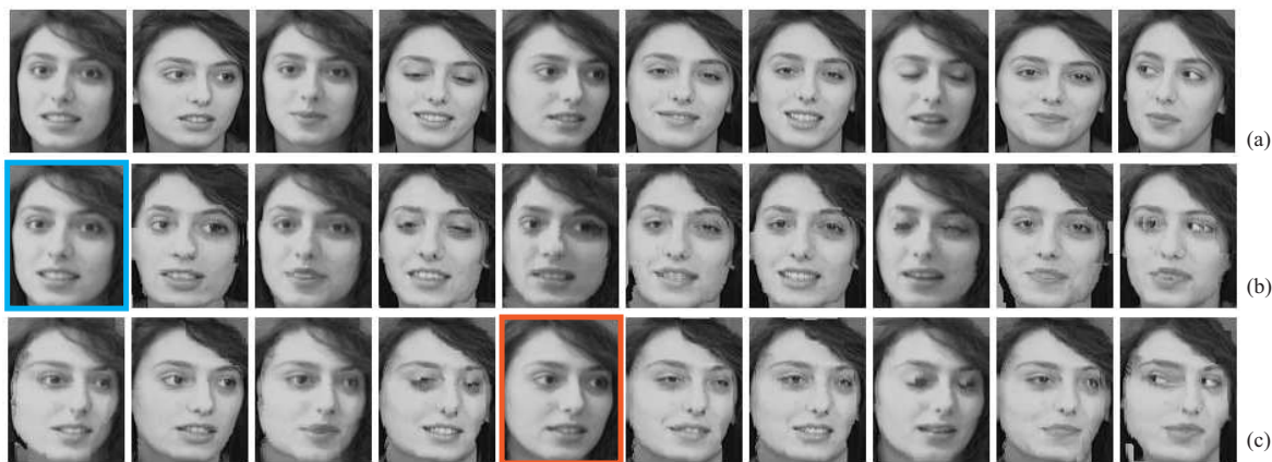
Fig. 23. SIFT flow can account for pose, expression and lighting changes for face recognition. (a): Ten samples of one subject in ORL database [44]. Notice pose and expression variations of these samples. (b): We select the first image as the query, apply SIFT flow to align the rest of the images to the query, and display the warped images with respect to the dense correspondence. The poses and expressions are rectified to that of the query after the warping. (c): The same as (b) except for choosing the fifth sample as the query.
