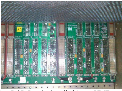
Figure 4 : Two ROD Panels, installed into a VME crate.
