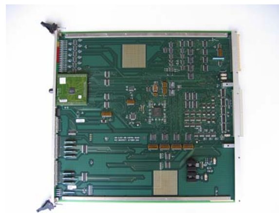
Figure 4: Clock and Control Board
