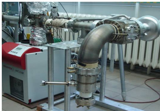
Fig.14. View of the UHV arc device with a truncated-cone cathode and the 90°-knee magnetic filter (without external windings), which was designed and constructed at IPJ in Swierk.
