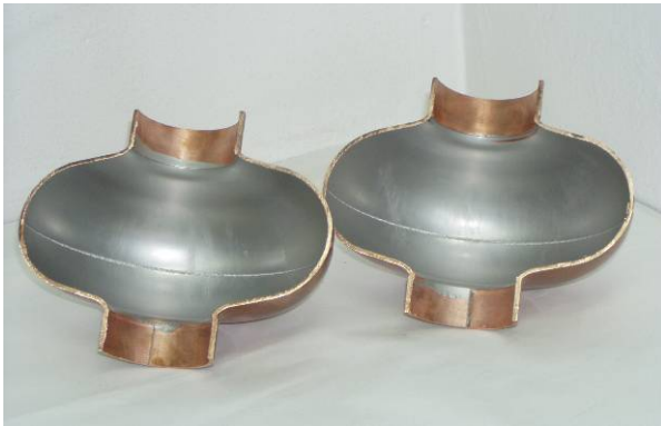
Fig.5. Photo of the model cavity, which demonstrates that the UHV arc facility with the cylindrical cathode can be applied for the deposition of a Nb-layer upon the whole inner surface.
