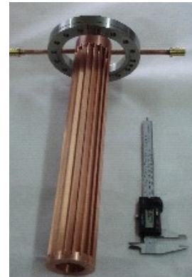
Fig.8. Picture of the Venetian-type filter designed for the UHV cylindrical arc facility.
