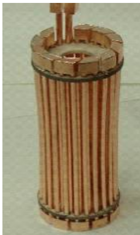
Fig.11. Picture of the prototype cylindrical filter consisting of thin tubes and appropriate connectors.
