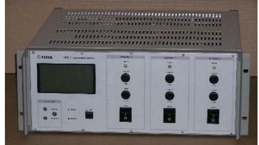
Figure 6: HPS1 200V DC power supply photo.
