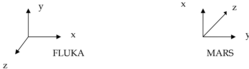
Figure 6: Right handed coordinate systems. The z axis coincides with the beam 1 axis, i.e the direction of the protons beam, coming out from the IP. With FLUKA, the x - y plane is seen from the end of the insertion, whereas with MARS, the y - x plane is seen from the IP.
