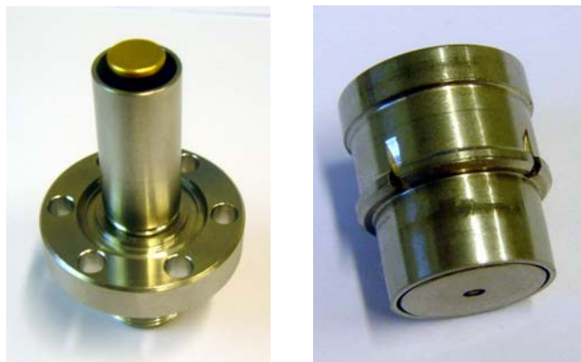
Fig. 14: These two pictures show different tested feedthrough from PMB, France. The left shows a gold plated stainless steel button with molybdenum conductor brazed to AL_2O_3 ceramic insulator. Usable directly mounting with the BPM body. The design is based on a
