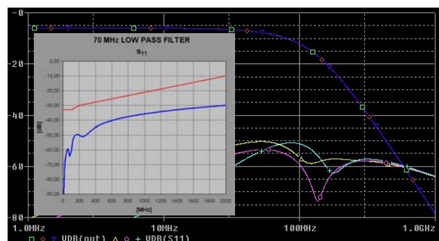
Figure 10: Parametric analysis using capacitor Cr and actual filter measurement. The red curve sets the upper limits of S11 during production.
