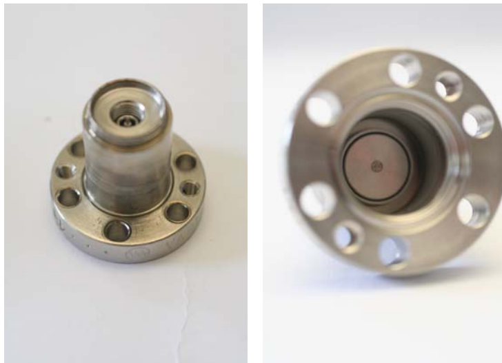
Fig. 11: PMB feedthrough, for welding construction, also welded to the test adapter
