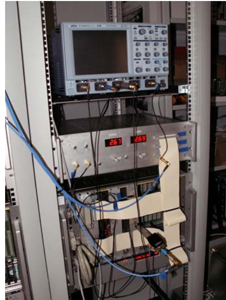
Fig. 3 Single bunch induced transient detection system
