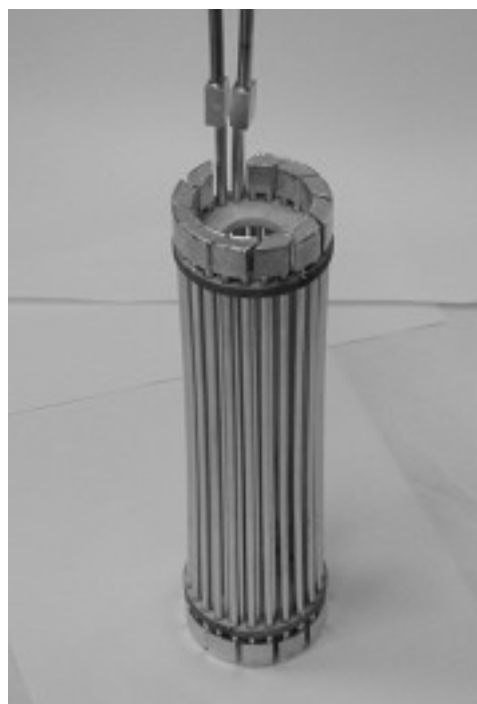
Fig. 9. General view of the cylindrical magnetic filter before its installation
