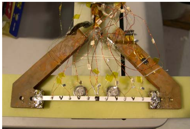
Fig. 5 Sample holder with HTS sample mounted for quench studies.
