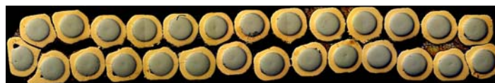
Fig. 2 Cross-section of the Nb 3 Al Rutherford cable. The packing factor of this cable is 90.1%.
