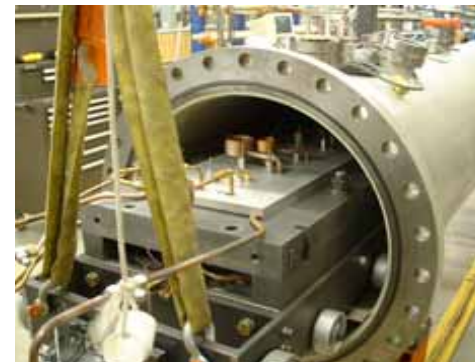
Coil in coffin, fitted for epoxy supply/purge, being inserted into retort
