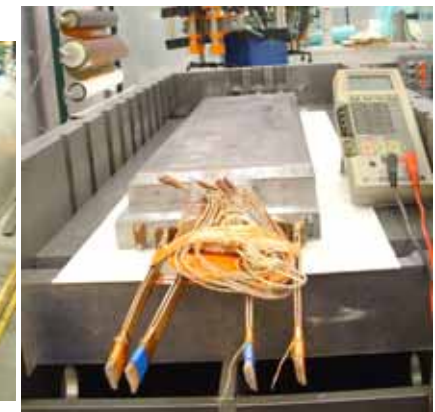
Impregnated coil with leads and test connections
