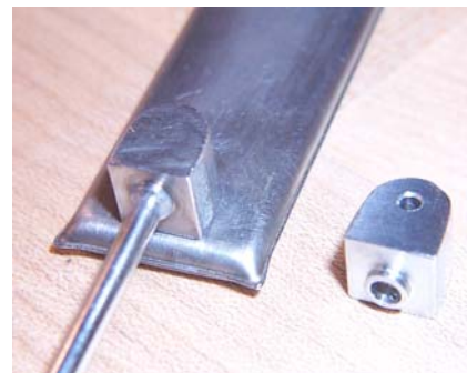
Fig. 4 Bladder with an inlet tube and housing. This design allows the manufacturer to laser weld the block to the top sheet of the bladder. After the block is attached, the top and bottom sheets can be laser welded together without the tube obstructing the machine path.
