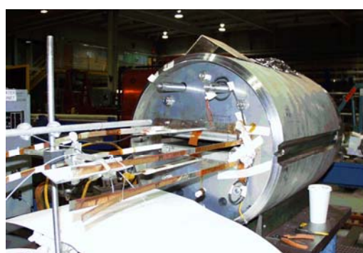
Fig. 7: React & Wind 32 mm aperture common coil dipole (left) that was recently built and tested at BNL. The magnet reached the computed short sample current (right).
