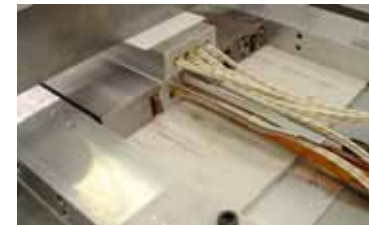
One joint assembled with heater module
