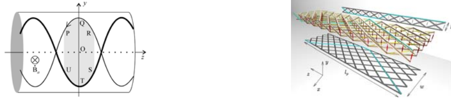
Fig. 1: Left: Sketch of filaments in a strand, courtesy of A. Verweij. Right: Electrical network representing a Rutherford-type cable, courtesy of R. de Maria.
