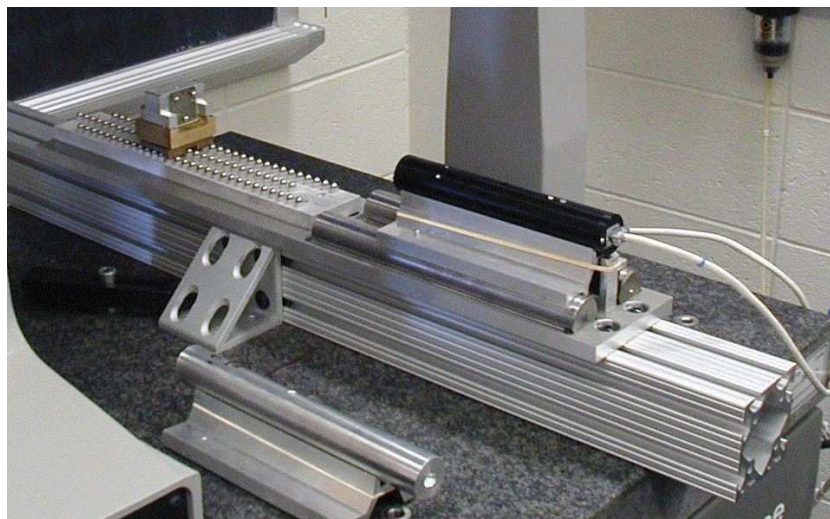
Figure 13. The calibration stand for the proximity sensors. This stand is used for calibrating both cameras and masks. It consists of a rail mount for the camera, and about thirty 3-ball mounts at different distances. Masks are mounted on a heavy brass interface-plate, which can be set on any of the 3-ball mounts.
