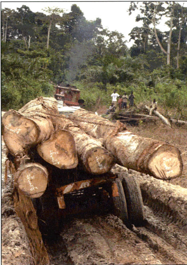
Figure 10: Logging truck passing through damaged section of road
