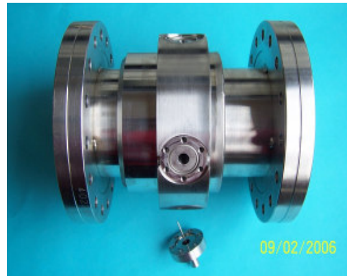
FIGURE 7: Drawing and photo of the modified BPM cavity.
