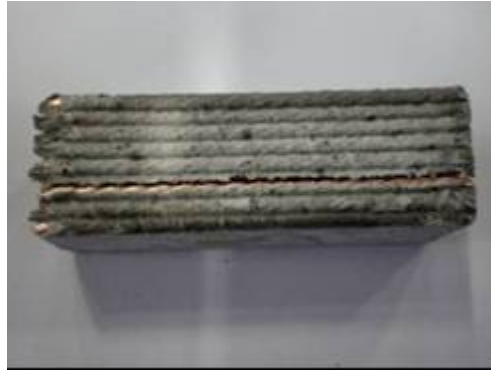
Fig.7: Stack of insulated cables reacted with a pre-compression, after outing of the reaction mould and relaxation of the cable stack
