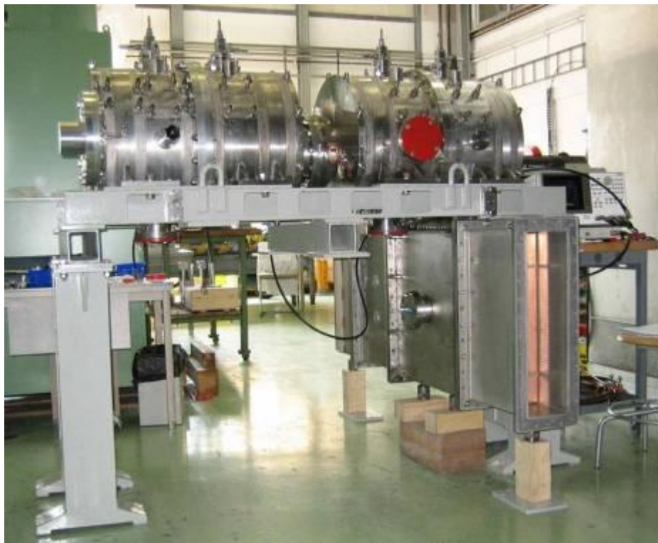
Figure 7 ISTC CCDTL prototype during low level measurements in the assembly area.
