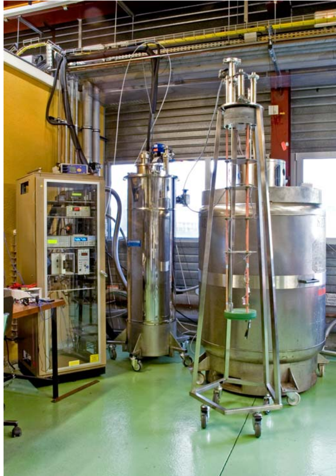
Figure 2. The NED facility at CEA Saclay. The automation and data acquisition system is located on the left. The cryostat itself is located in the middle of the photo and on the right side of the picture one can see the insert with the lambda plate (green piece).
