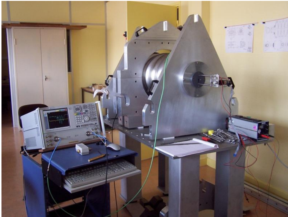
Figure 2: bead-pull setup on the cavity tuning bench
