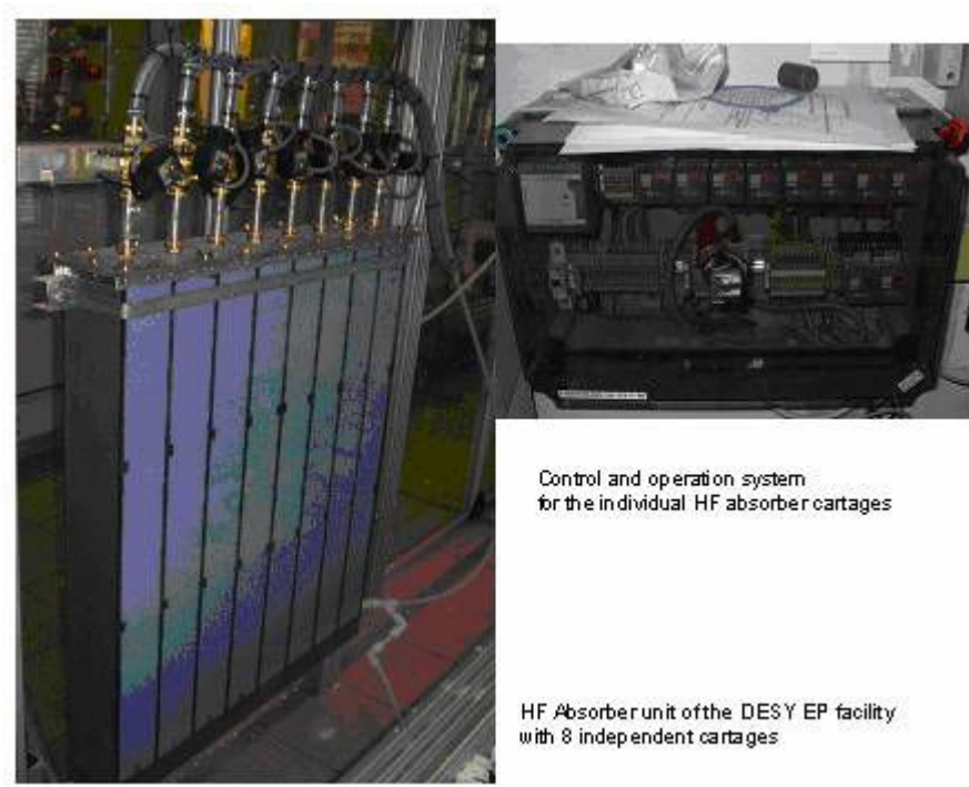
Fig. 8: Picture of the new development of gas scrubber for HF exhausting gasses
