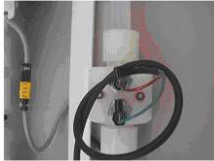
EP U/I test cell integrated into the EP acid line towards the cavity
