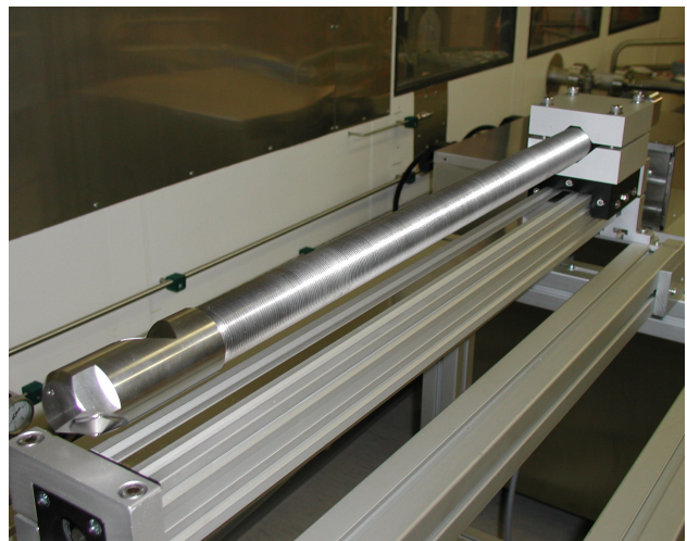
Figure 2: CO 2 - cooler/purifier unit (left) and horizontal motion unit with the spraying cane assembled on the linear drive (right)
