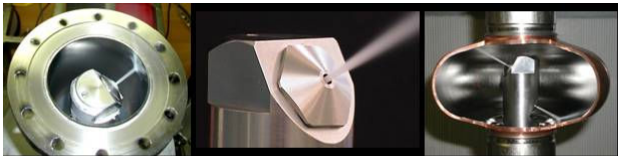
Figure 5: Commissioning of the dry-ice system: Optical checks of the jet under different conditions
