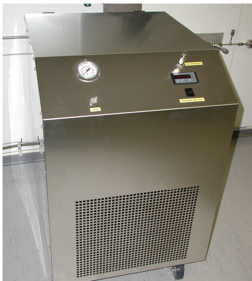
Figure 2: CO 2 - cooler/purifier unit (left) and horizontal motion unit with the spraying cane assembled on the linear drive (right)
