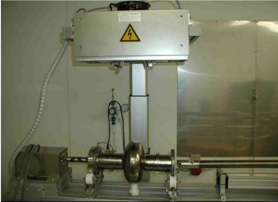
Figure 3: Dry-ice cleaning system with the new IR heater
