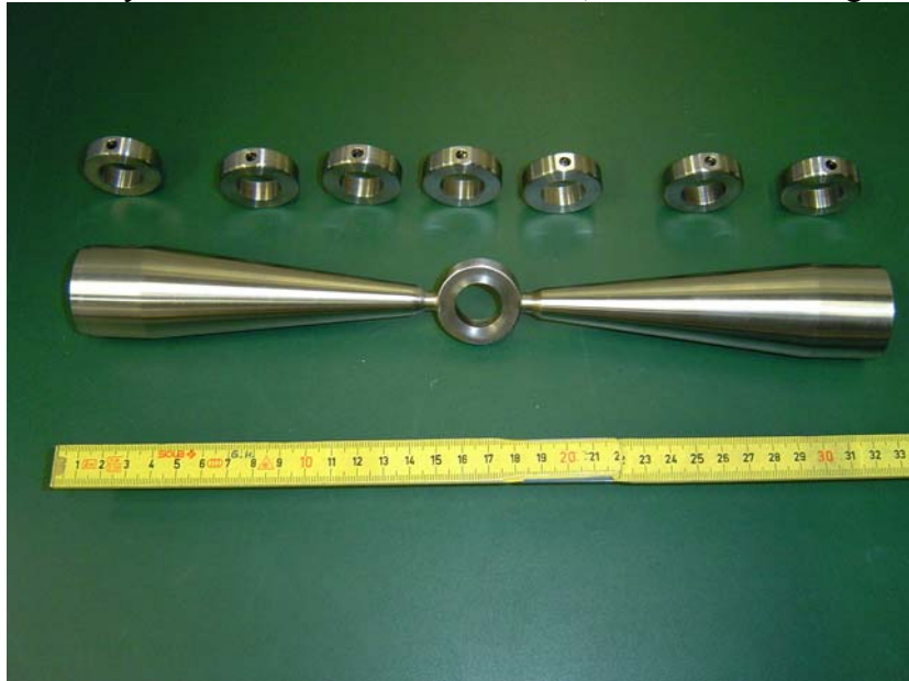
Fig.8: a view of one stem with the central rings: it is possible to notice the aperture for the cooling water.
