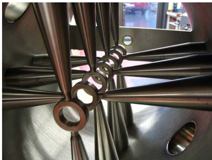
Fig.10: The inner part of the cavity after welding.
