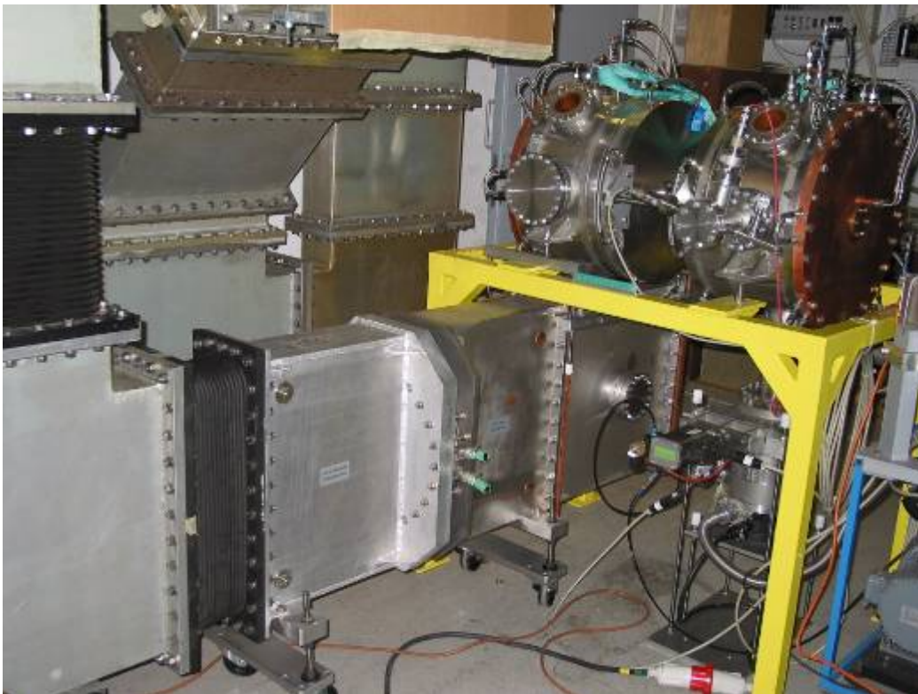
Figure 7 CCDTL in the high power stand connected to the wave guide ready for high power test.
