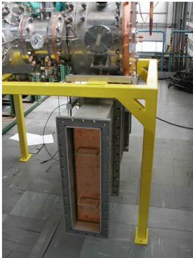
Figure 11. Mechanical set-up for waveguide to cavity coupling measurements
