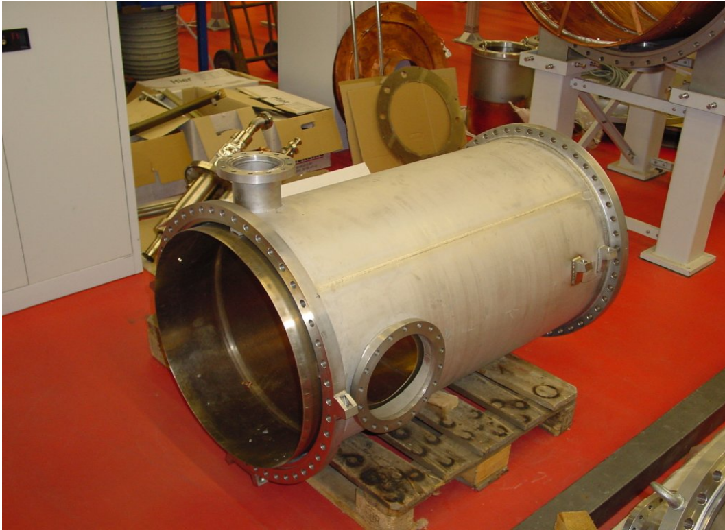
Figure 22: Main part of the cold mass with magnetic shielding inside
