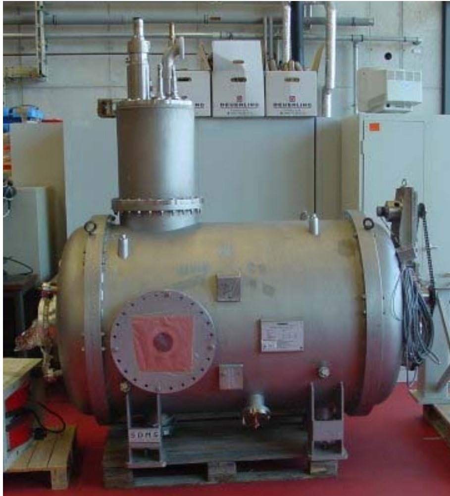
Figure 19: Cryomodule with tuning possibility for operation in horizontal position
