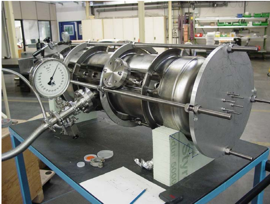
Figure 6: The CH-cavity during a vacuum test before the chemical treatment
