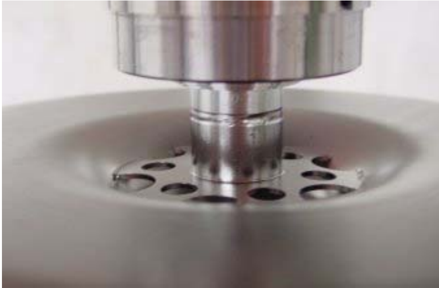
Figure 16: Connection between outer drift tube and corpus of the cavity
