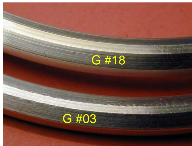
Figure 14: photos of gasket #18 and gasket #03 after the compression cycles.
