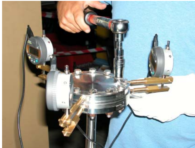
Figure 22 : manually compression test using a torque meter on the bolts head: the leak detector is connected to the bottom flange.
