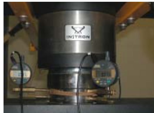
Figure 6: a particular of the flanges in the test machine and the electronic gauges applied to them.
