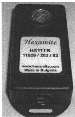
Figure 5: Hexamite Hx11 ultrasonic positioning device module [10].
