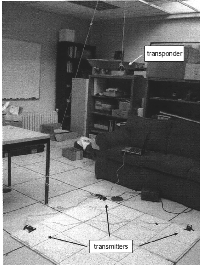
Figure 13: experimental set up with three transmitters and one transponder.
